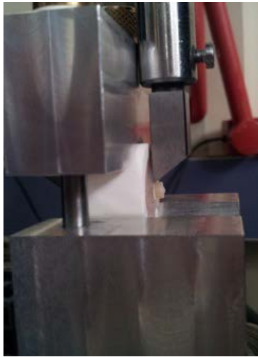
Figure 2. Shear bond strength testing apparatus
