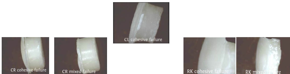
Figure 5. View of the failure type for porcelain substrates
