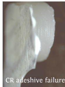
Figure 4. View of the failure type for metal substrates
