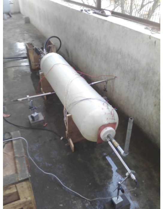
Figure 4. Composite pressure vessel filled with water and subjected to hydraulic pressure for hydraulic test
