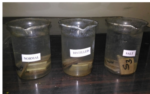
Figure 4. Test specimens immersed in normal, distilled and salt water
