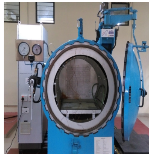
Figure 1. Fabrication of composite laminates using vacuum bagging process and post-cured using autoclave machine
