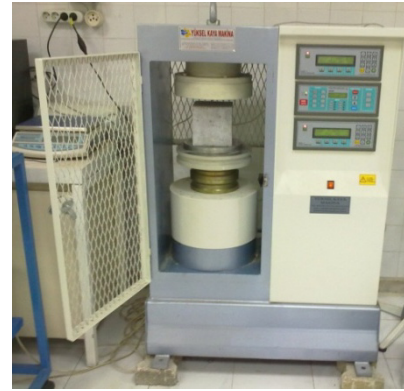
Figure 2. Testing of compressive strength test specimen
