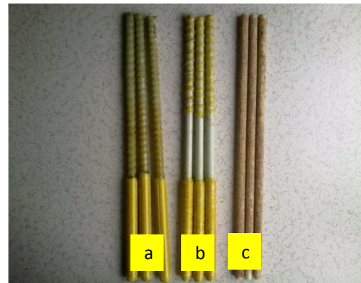
Figure 1. Glass fibre reinforced polymer (GFRP) rebars a) helically deformed b) ribbed c) sand coated
