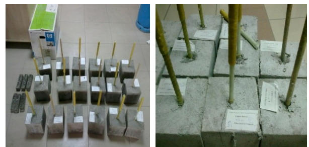
Figure 6. Pull-out test specimen positioned on testing equipment
