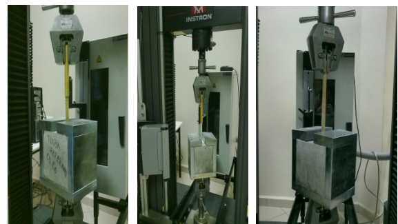
Figure 7. Pull-out test specimens before and after experiment
