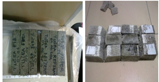
Figure 4. Reference and Aramid fibre-reinforced samples before (a) and after (b) test
