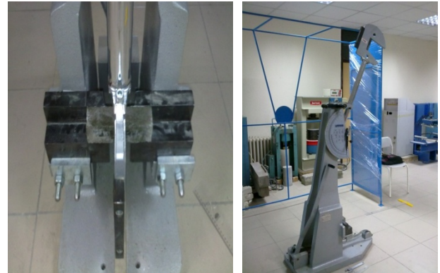
Figure 3. Testing of Impact Charpy strength test specimen
