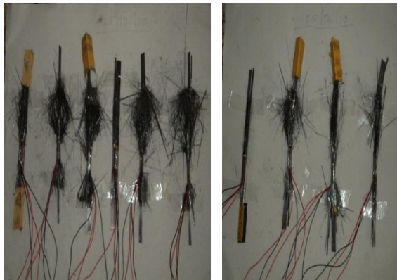
Figure 17. Failure mode s of longitudinal Tensile Specimens
