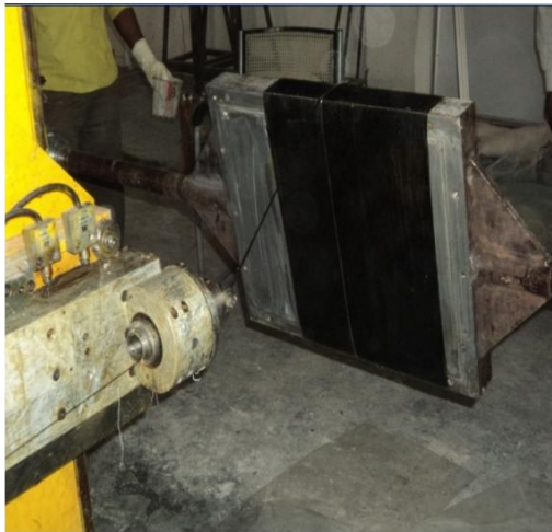
Figure 2. Filament winding Process using Towpreg on flat Mandrel
