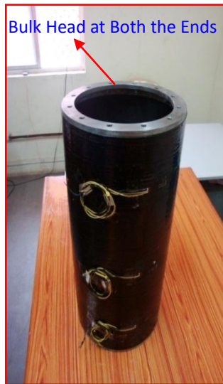
Figure 43. Composite shell with end Bulkheads and Strain Gauges
