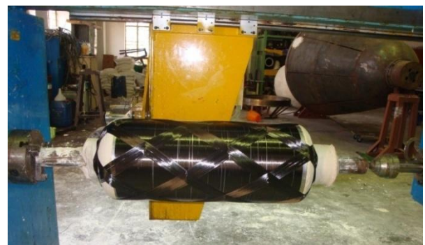
Figure 40(a). Helical winding
