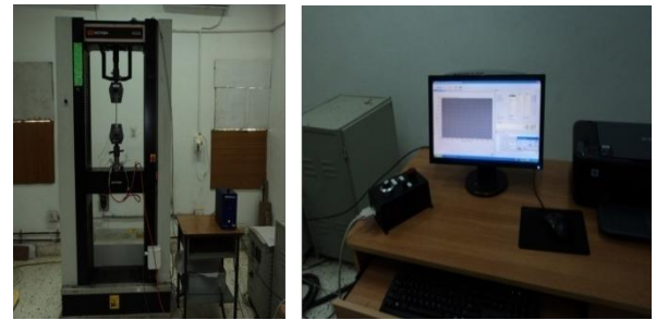
Figure 15. UTM - 100KN Capacity with strain data acquisition system
