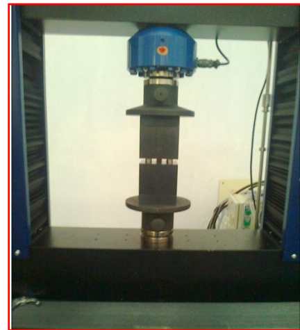
Figure 18. IITRI test fixture for compression
