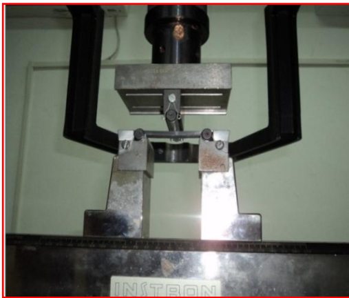
Figure 21. 3 point flexural testing
