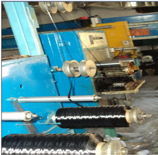
Figure 1. Mounted Towpreg spools
