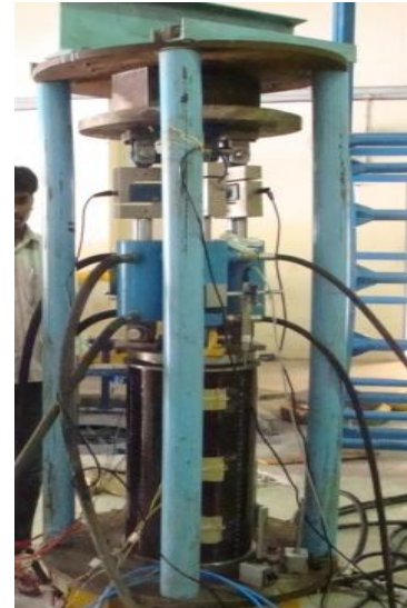
Figure 44. Test Rig and Composite Cylinder Setup
