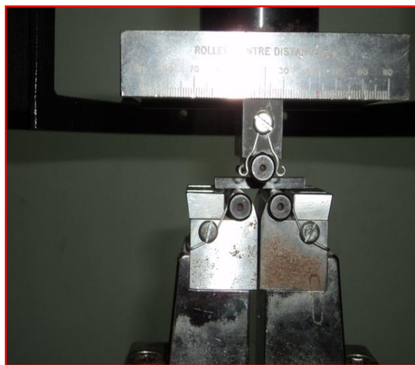
Figure 24. ILSS Testing
