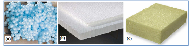
Figure 3. Schematic of the cellular cores, (a) YmaCell, (b) poplypropylen honeycomb and (c) AIREX thermoplastic foam
