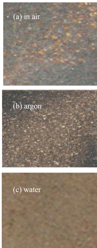
Figure 6. Photo images of LASER etched area of WPC in (a) air, (b) argon and (c) water
