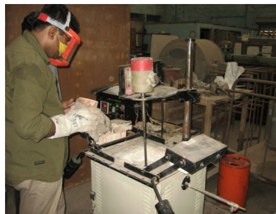
Figure 2. Experimental set up for fabrication of aluminum metal matrix composite
