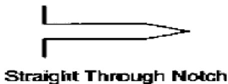
Figure 6. Fatigue crack starter notch configuration
