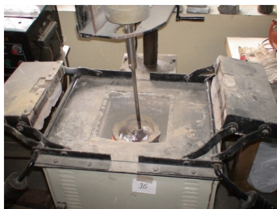
Figure 1. Experimental set up for processing of AA2024/fly ash composites
