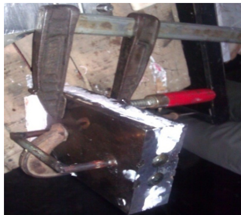
Plate 3. Curing of the epoxy resin-foundry slag particulate blend
