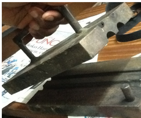
Plate 2. A medium carbon basic die mould with improvised cavity
