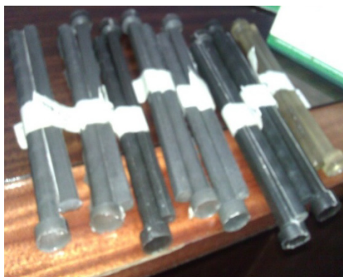
Plate 4. Cast ingots of the epoxy resin-basic slag particulate composite
