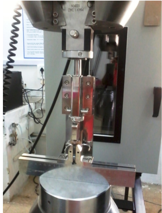
Figure 15. Inter-laminar shear strength measurement as per ASTM D-2344
