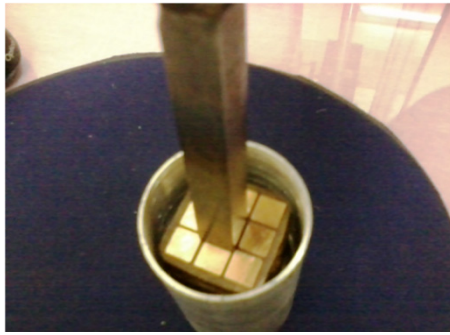
Figure 12. Test set up for shear strength measurement
