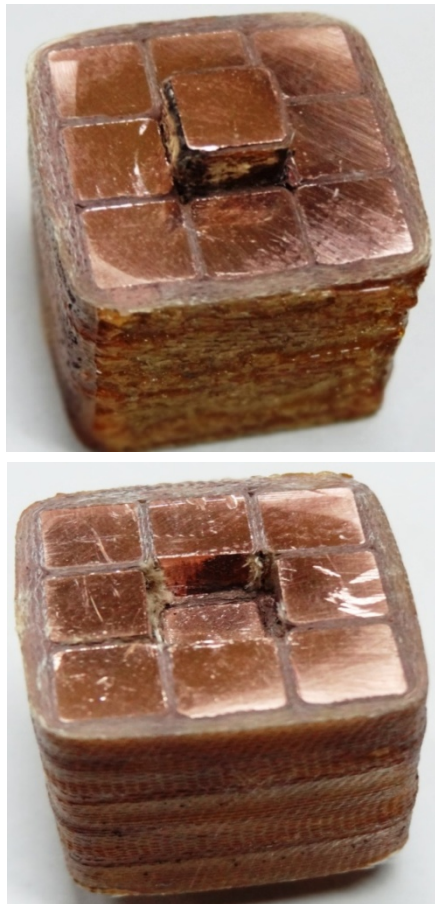
Figure 13. Shear test sample as copper sliding out of array
