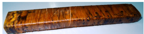
Figure 16. Array tested for Flexural strength measurement
