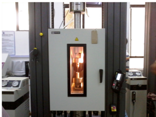
Figure 14. Shear strength measurement of array at 350 C
