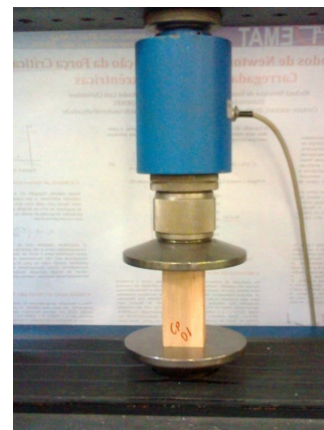
Figure 5. Compression test parallel to grain accomplished with the aid of the universal testing machine EMIC MEM 10000
