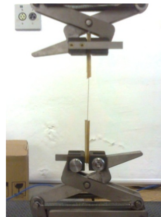
Figure 9. Testing machine EMIC DL 500 used in the tensile test
