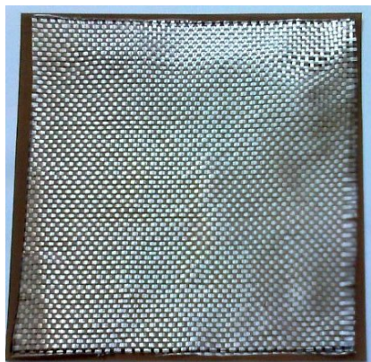
Figure 7. Woven glass fiber used in the manufacture of the laminate composite
