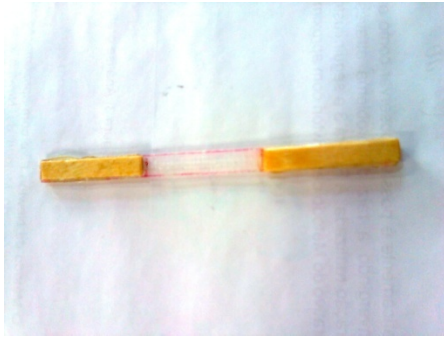
Figure 10. Specimens of laminate composite for tensile tests
