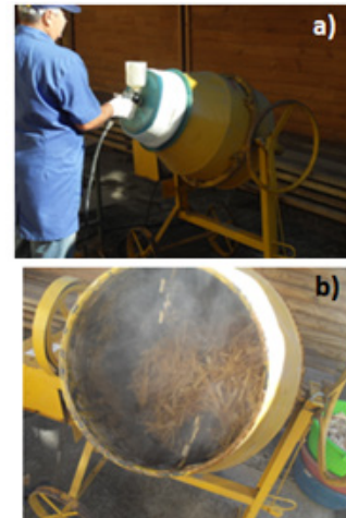
Figure 2. Resin application (a) and strands getting out gluing equipment (b)
