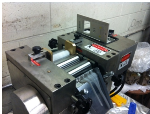
Figure 4. The three-roll mill equipment used in the calendaring process
