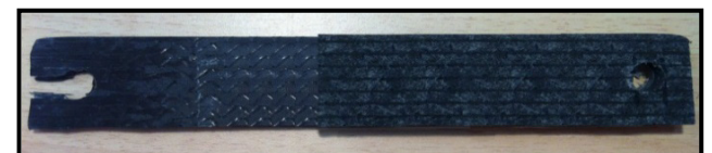
Figure 11. Tearing-off problems in SLJs that were without quasi-isotropic tabs as a result of being subjected to the highrate loading
