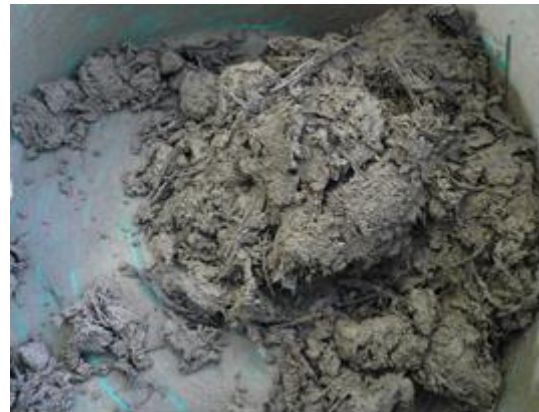
Figure 1.1. AR glass fiber concrete mix
