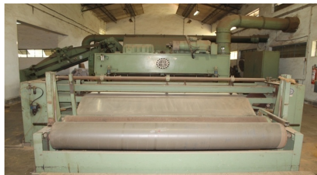
Figure 4. Besch NR_51 needle punching machine
