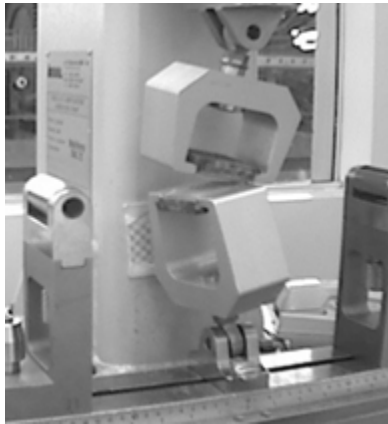
Figure 6. Perpendicular tensile test
