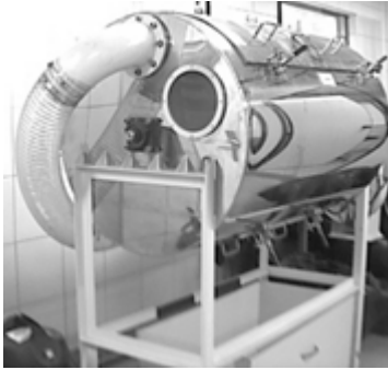
Figure 1. Cylinder to mix fiber and resin
