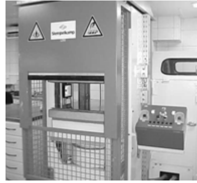
Figure 4. Machine to press the board with control of pressure and temperature
