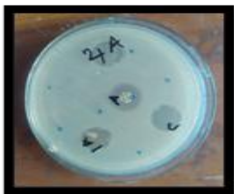
Figure 3. Antibacterial study of the Cu(salen): The bacteria is Shigella Sonnei and the media is Muller Hinton agar. 1A and 4A are Cu(salen) dimer complex, A is antibiotic streptomycin disk, C is \text{CHCl}_3
