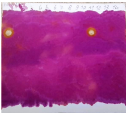
Image of ethylene glycol chromatogram and Liq1-14. Silica gel plate on aluminium; Eluant: 90% butan-2-ol, 9% distilled water and 1% glacial acetic acid; Developer: Potassium permanganate solution; Ethylene glycol R_f = 0.7 .
