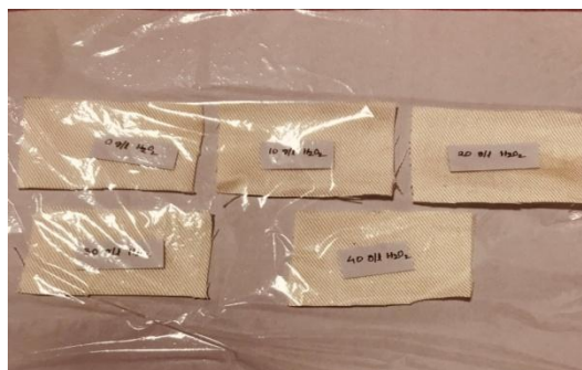
Figure 1. Grey Cotton Twill Fabric Saturated with Different Concentration of Hydrogen Peroxide
