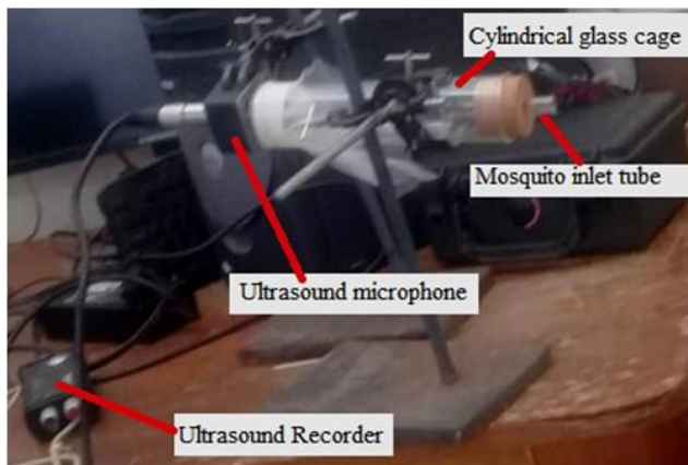
Figure 1. The sound recording setup
