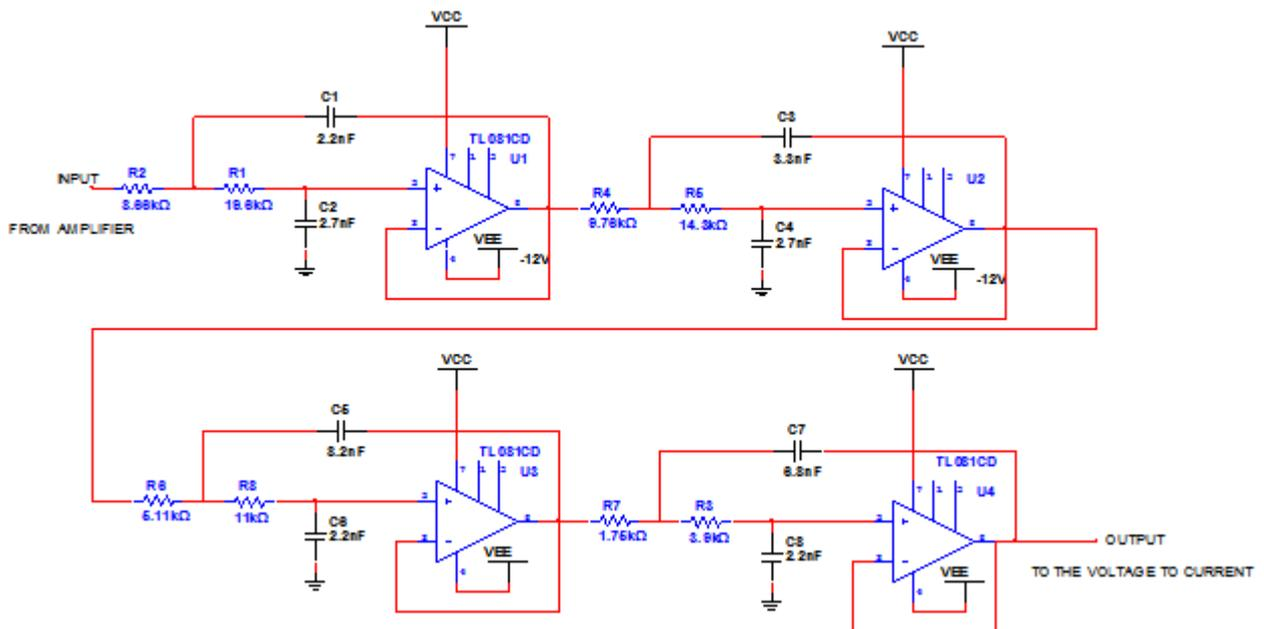
Figure 3. 8<sup>th</sup> order Butterworth filter of transducer unit
