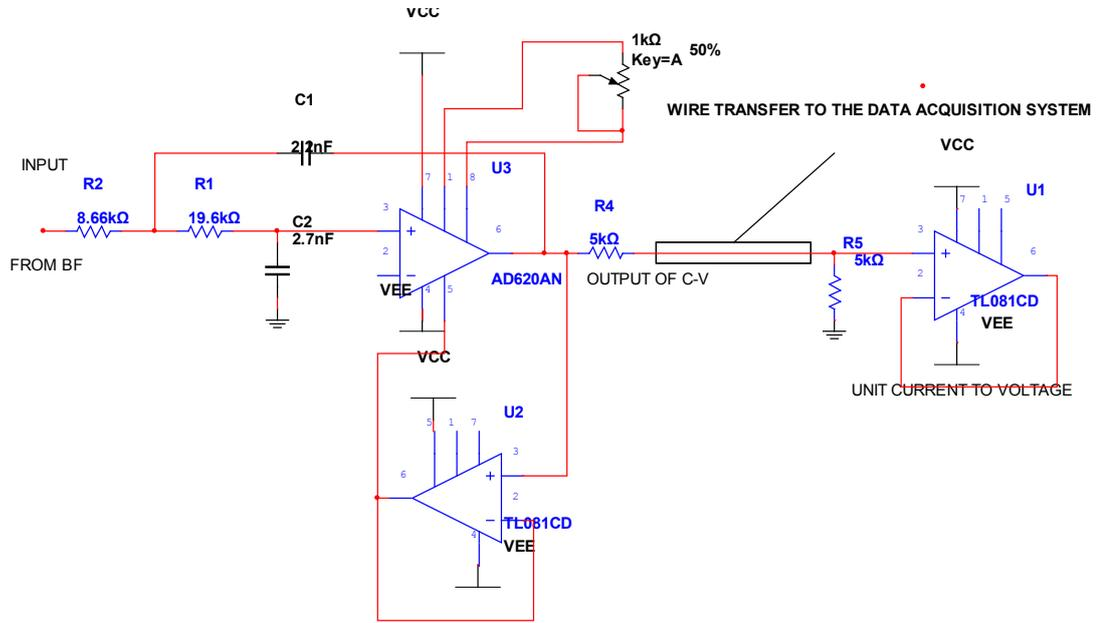
Figure 4. Voltage to current circuit of transducer unit
