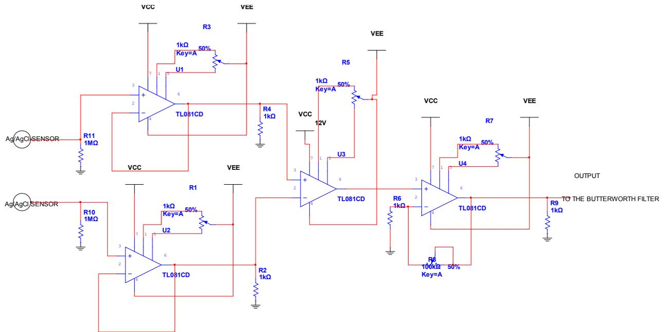
Figure 2. Interface and amplifier circuit of transducer unit
