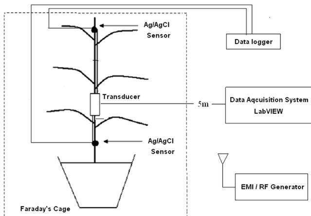
Figure 5. The experimental system for the measurement of plant’s signal
