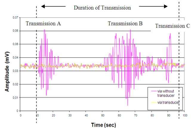
Figure 6. The effect of EMI testing in transmission of signal via direct connection of sensor to data logger (-) and via transducer unit (-)
