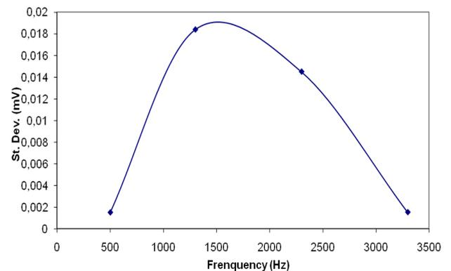
Figure 7. Standard deviation of signals by effect of EMI testing
