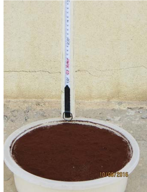
Figure 1. Tape measure fixed with plastic tube to the vertical side
