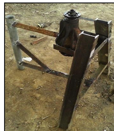
Plate 3. The Seating for the Motor Axel with the Axel Mounted
