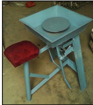
Plates 8. a & b. The Axel (Potter's) Kick Wheel
