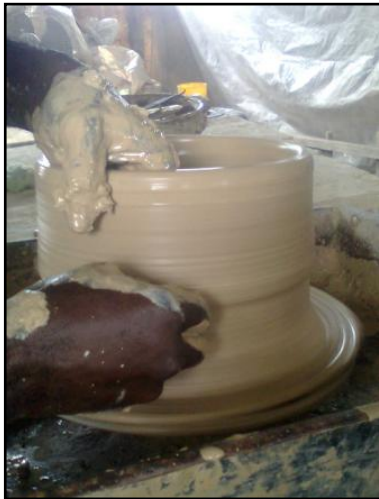
Plate 9. The machine is powerful enough to center large lumps of clay
