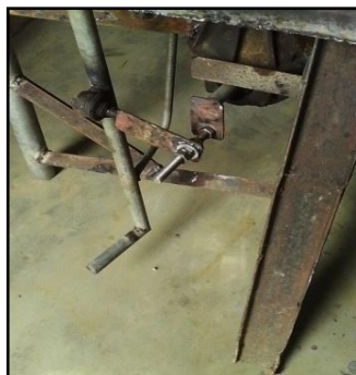
Plate 5. The Assembly of the Foot Pedal
