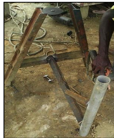
Plate 2. Framework and Stand for the Wheel
