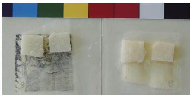
Figure 9. Agar-lipase gel system application on mock-ups verso side to activate tape adhesive glue
