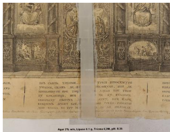
Figure 11. Agar 2% w/v-enzyme lipase gel system application on the oxidized glue residue deposition
