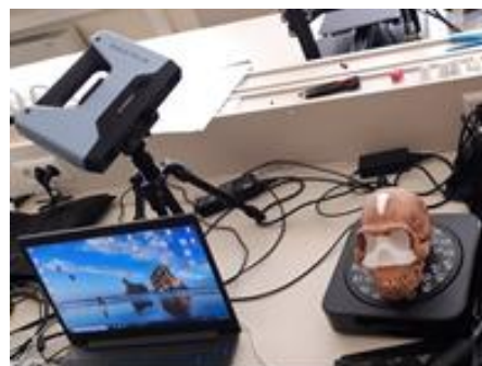
Figure 1. Experimental setup used to measure the cranium in 3D
