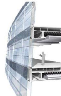
Figure 4. High Performance Active Facade Detail of Pearl Tower
