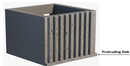
Figure 10. Shows the protruding slab where molds are laid and loads of the bricks are carried
