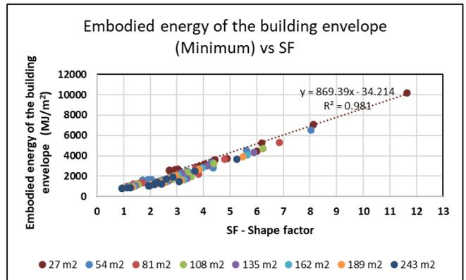
**Figure 12.** Embodied energy of the building envelope (minimum) vs. SF for different floor areas of a building
