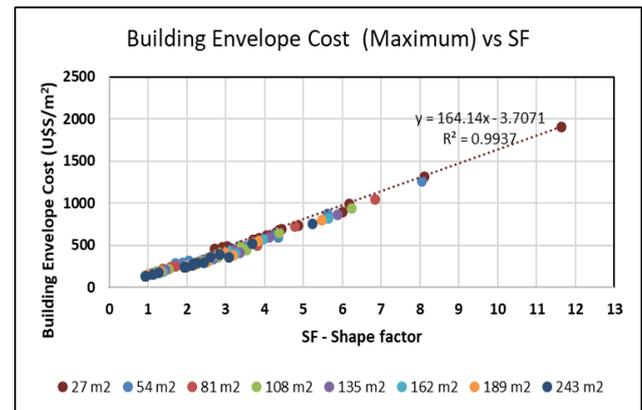
**Figure 9.** Building envelope cost (maximum) vs SF for different sizes of floor area of a building
