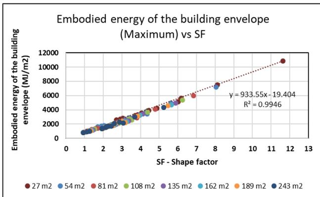
**Figure 11.** Embodied energy of the building envelope (maximum) vs. SF for different floor areas of a building
