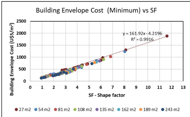
**Figure 10.** Building envelope cost (minimum) vs SF for different sizes of floor area of a building
