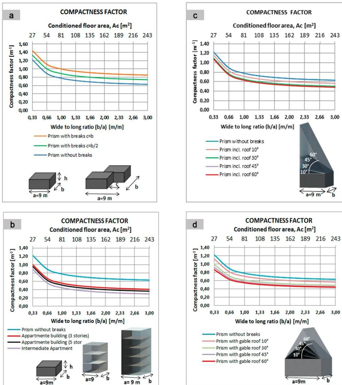
**Figure 8.** CF of building for: floor plan variations (Fig 8a); different number of floors (Fig. 8b); with mono-pitched roofs (Fig 8c) and with gabled roofs (Fig. 8d), these for tilt angle from  $10^\circ$  to  $60^\circ$
