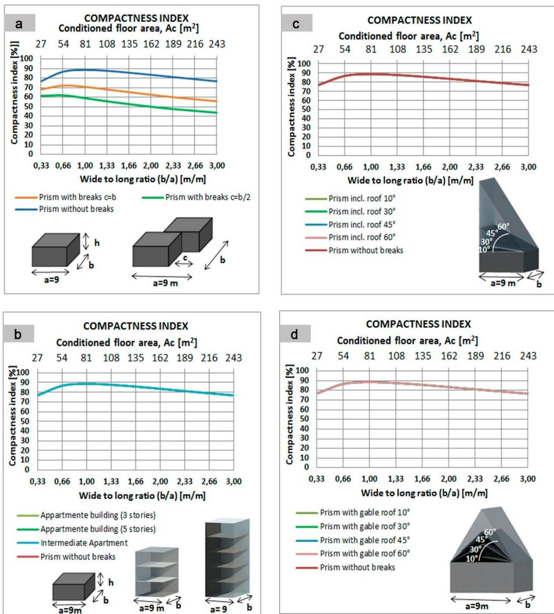
Figure 7. CI of building for: floor plan variations (Fig 7a); different number of floors (Fig. 7b); with mono-pitched roofs (Fig 7c) and with gabled roofs (Fig. 7d), these for tilt angle from  $10^\circ$  to  $60^\circ$
