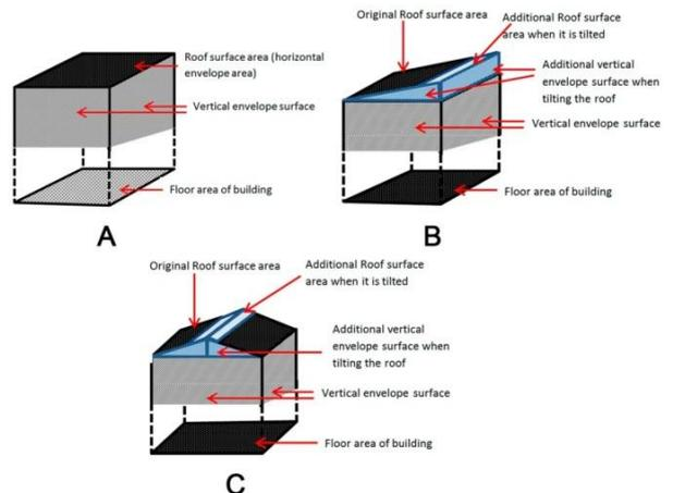
Figure 4. Prism and roof: 4A. Prism without breaks and an horizontal roof, 4B. Building with mono-pitched roof, 4C. Building with dual-pitched roof or gable roof
