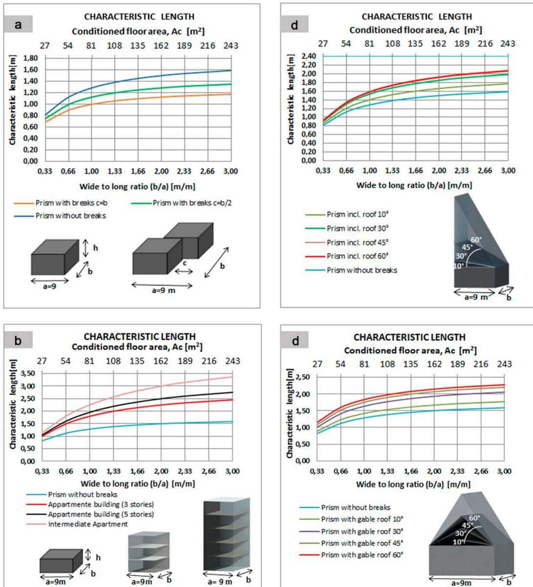
**Figure 6.** CL of building for: floor plan variations (Fig 6a); different number of floors (Fig. 6b); with mono-pitched roofs (Fig 6c) and with gabled roofs (Fig. 6d), these for tilt angle from 10° to 60°
