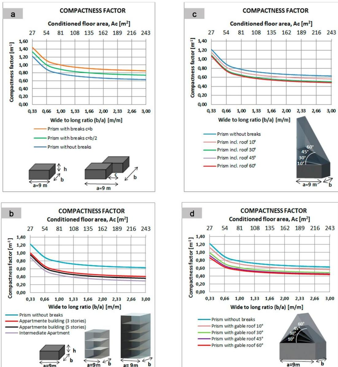
**Figure 5.** CF of building for: floor plan variations (Fig 5a); different number of floors (Fig. 5b); with mono-pitched roofs (Fig 5c) and with gabled roofs (Fig. 5d), these for tilt angle from  $10^\circ$  to  $60^\circ$
