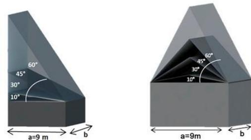
Figure 3. Mono-pitched roof and the dual pitched roof or gable roof from 10° to 60°
