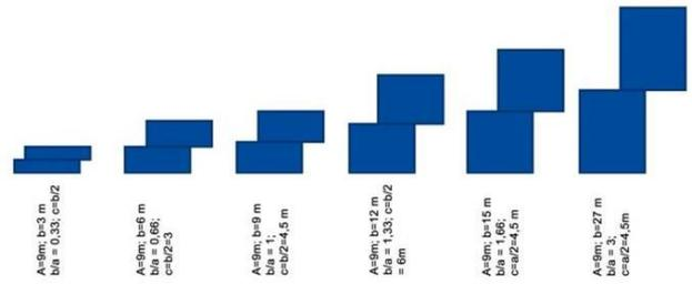
Figure 2. Variation in floor plans when there are sectional breaks which can generate more vertical envelope surface
