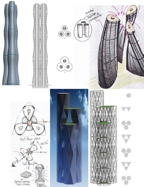
Figure 6. Left: Wave-form tower cluster (Land.P,[5]); Wind and light flows through openings thus reducing wind loading on tower clusters. Middle: Clustered towers for wind harvesting (Seyedinnoor, 2011, [4]); taper, twisted, curved corners, aerodynamic, funnel effect and wind turbines-equipped. Right: triangulated mega frame structure (Land. P,[5]); Clustering of the structure Pyramids allow a flexible articulation of the overall clustering form giving interior atria and through space
