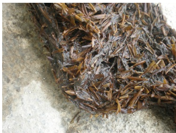
Figure 2. Picture of rice husk package with attached biomass after 3 months operation
