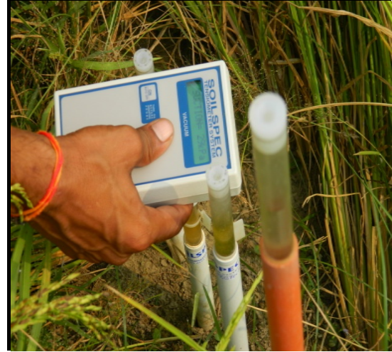
Figure 2. Soil spec in action measuring soil water tension
