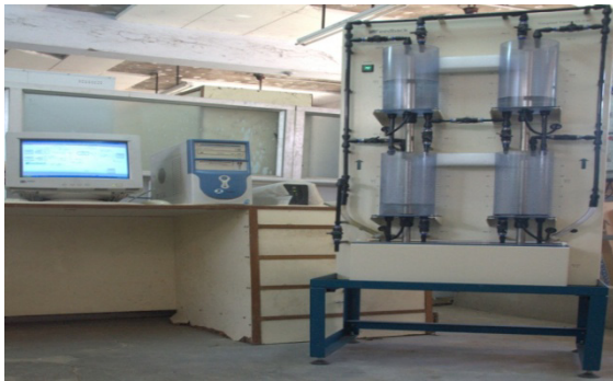
Figure 5a. Experimental setup for two interacting tank level control system
