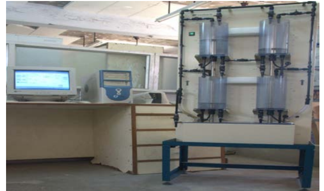
Figure 5a. Experimental setup for two interacting tank level control system
