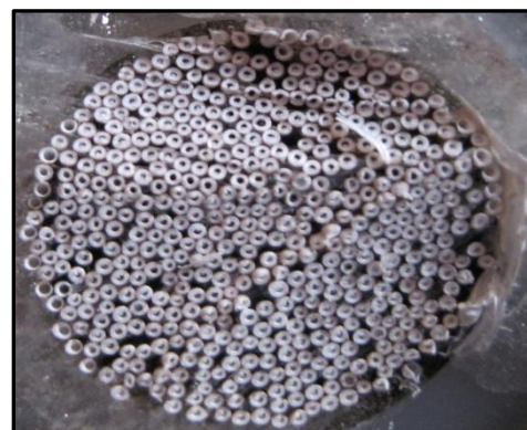
Figure 1. Cross section of the fabricated high pressure stainless steel module
