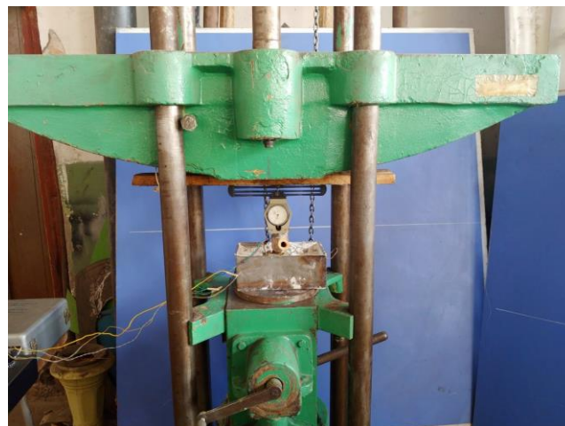
Figure 11. General view of the installation of the universal testing machine UIM-50
