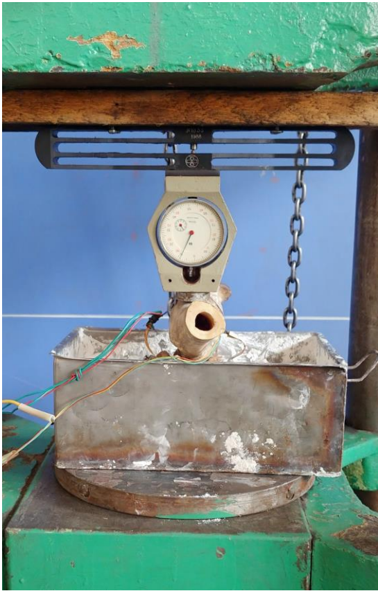
Figure 12. The test object with the dynamometer DOSM-0.2-10
