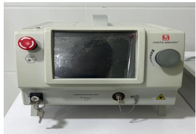
Figure 1. Surgical laser "LAKHTA-MILON" - laser device for phlebology
