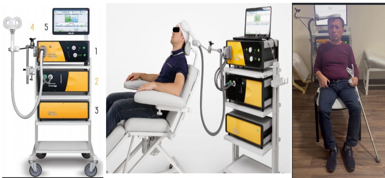
Figure 3. Equipment overview and transcranial magnetic stimulation procedure. Transcranial magnetic stimulator (Neuro-MS/D) 1 – main unit; 2 – cooling module; 3 – charging module; 4 – inductor bracket; 5 – display and programs
