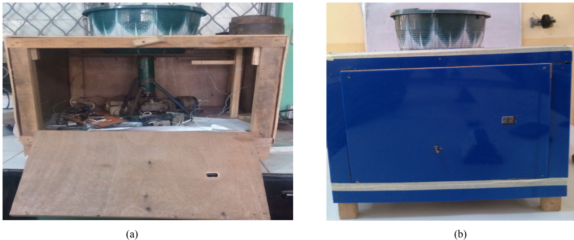
Figure 8. Picture of the designed electromechanical speed control system (a) interior view and (b) completely cased system
