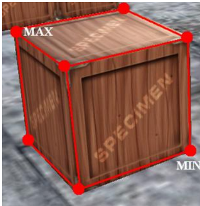
Figure 4. Bounding box with its minimum and maximum points
