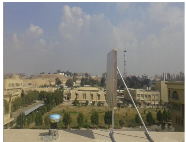
Figure 3. Vertical reflecting panel (1mX1m). away 1m from the receiver(Rover)
