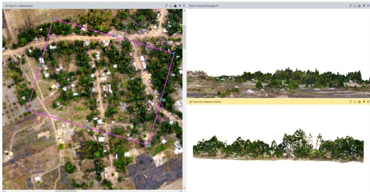
**Figure 9.** Sample photogrammetric point clouds displayed using ERDAS Imagine Point Cloud Tools. Clockwise from left shows the selected area; its 3D representation and a side view profile
