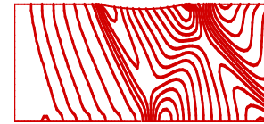
Figure 29. Mach contours (Jameson) inlet M=1.4 k^4 = \frac{1}{10059} , k^2 = \frac{1}{75}
