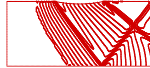
Figure 18. Mach contours (Jameson) inlet M=1.65
