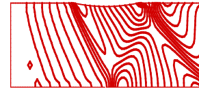
Figure 30. Mach contours (Jameson) inlet M=1.4 k^4 = \frac{1}{10049} , k^2 = .6
