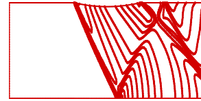
Figure 9. Mach contours (TVD) inlet M=1.4
