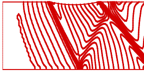
Figure 25. Mach contours (Jameson) inlet M=1.4
