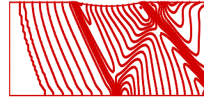
Figure 8. Mach contours (Jameson) inlet M=1.4
