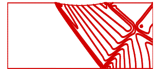
Figure 21. Pressure contours (Jameson) inlet M=1.65
