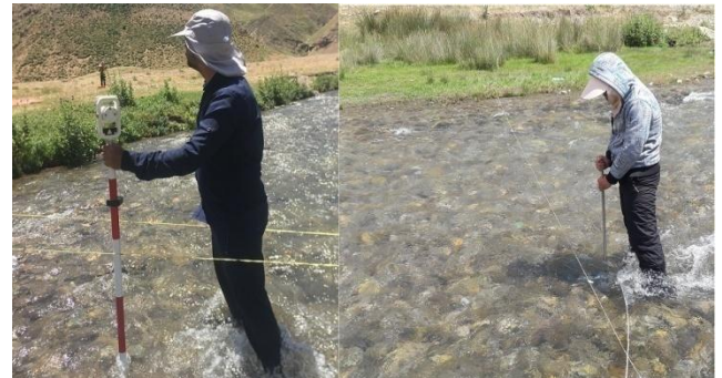
Figure 4. Velocity measurement in the reach with vegetated banks
