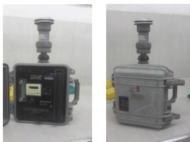
Figure 2. A MiniVol Tactical Air Sampler (TAS) [28]
