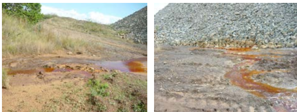
Figure 3. Acid Mine Drainage (AMD) from Waste Rock piles at Nyabigena draining to the Environment (Source: [13])
