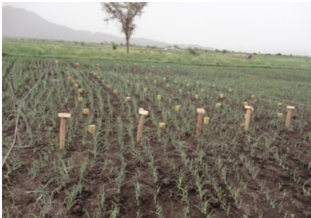
Figure 2. Sample collection using catch cans: at sprinkler system
