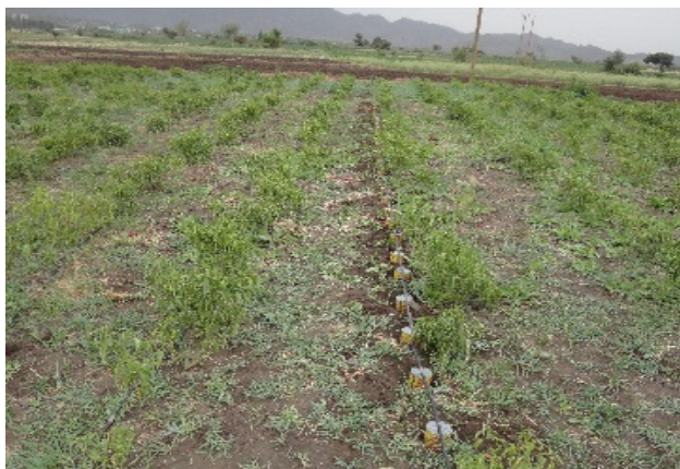
Figure 3. Sample collection using catch cans: at drip system
