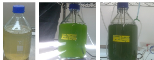
Figure 1. Acclimatizing algae to municipal wastewater
