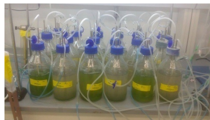
Figure 3. Experimental setup for treatment of wastewater by Chlorella
