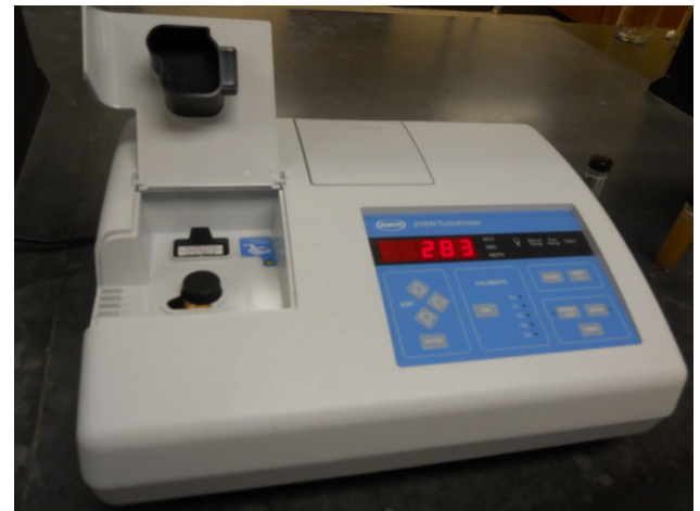
Figure 1. Turbidity measuring device
