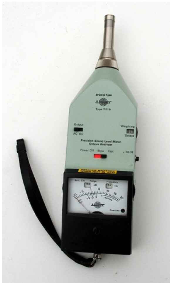
Figure 1. Bruel & Kjaer (Type 2215) Precision Sound Level Meter
