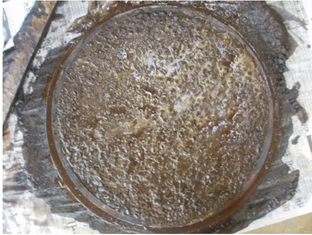
Figure 4. Wet track abrasion test of microsurfacing mix
