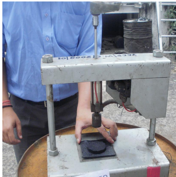
Figure 3. Cohesion Test of microsurfacing mix
