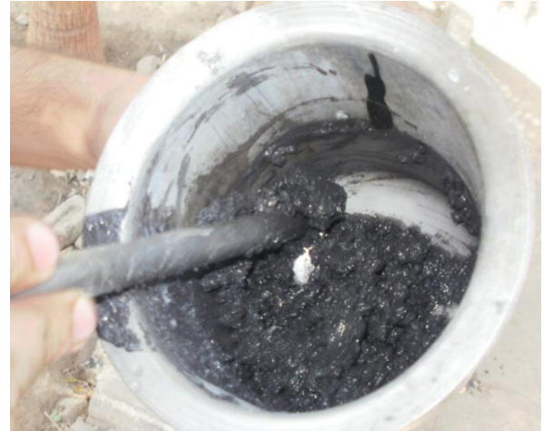
Figure 2. Manual mixing test of microsurfacing mix
